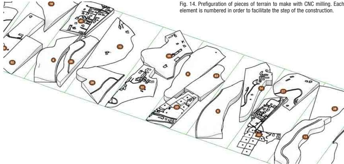
Fig. 14. Prefiguration of pieces of terrain to make with CNC milling. Each element is numbered in order to facilitate the step of the construction.
