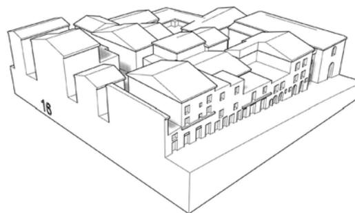
Fig. 11. Modular grid for the discretization of the historic centre and the creation of 15 x 15 cm size blocks.
