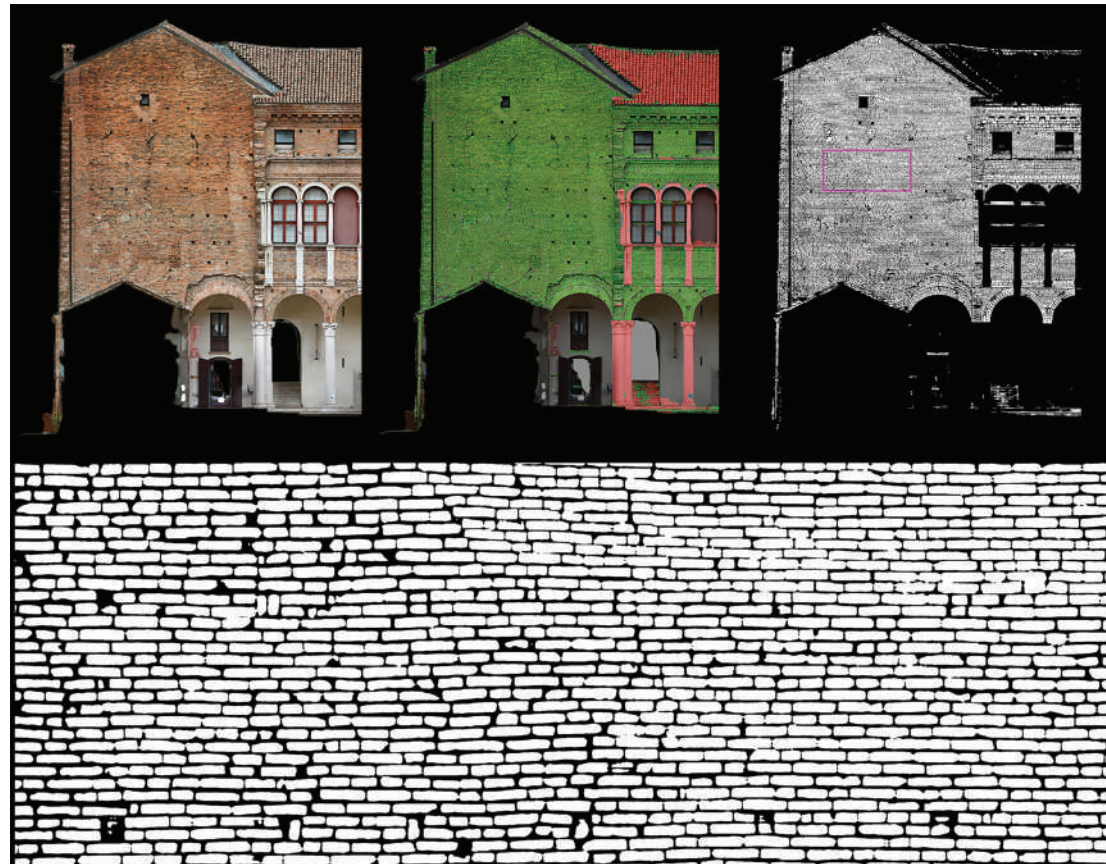
Figure 9. The brick mask obtained from algorithmic processing, if critically interpreted, can support the reading of surface features. In the case of the main façade of the building, on the west elevation facing the Cortile d'Onore , a diagonal trace emerges, formed by the alignment of several vertical mortar joints. Starting from the junction between the main façade and the roof, this feature extends continuously for approximately 9.8 m. Graphic elaboration by the authors.
