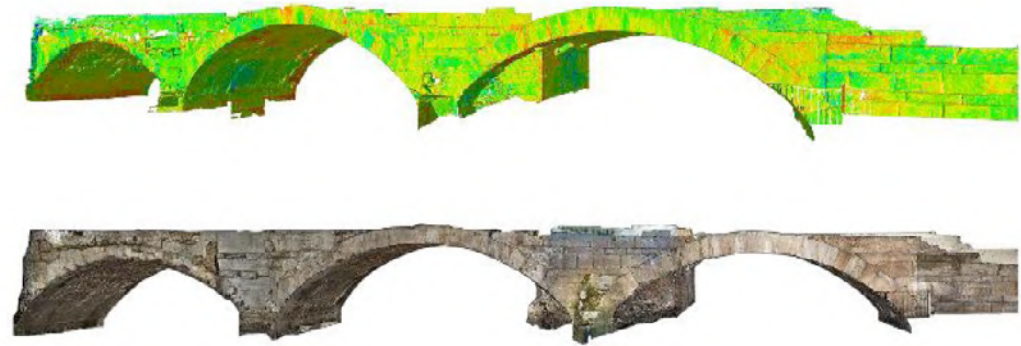
Fig. 1 - The point clouds of a bridge generated by laser scanning (above) and by SfM (below).
