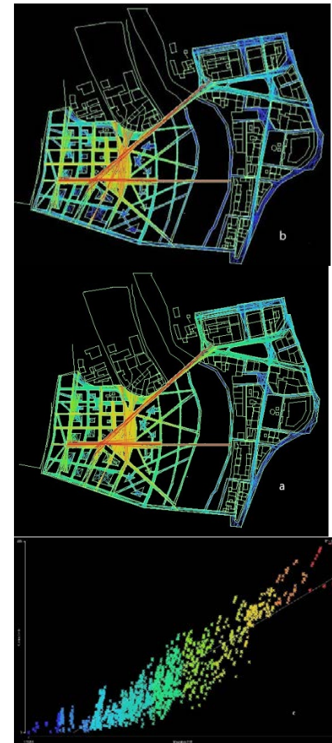
Fig. 12 – a) Connectivity and b) integration results maps. c) Intelligibility score 0.87 (Merzouk and Chebila, 2020).
