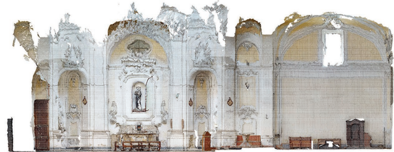
Fig. 10 - Point clouds of the interior sections of the church from the laser scanner acquisitions. Survey by Mario Ronca, supervisor Manuela Piscitelli.
