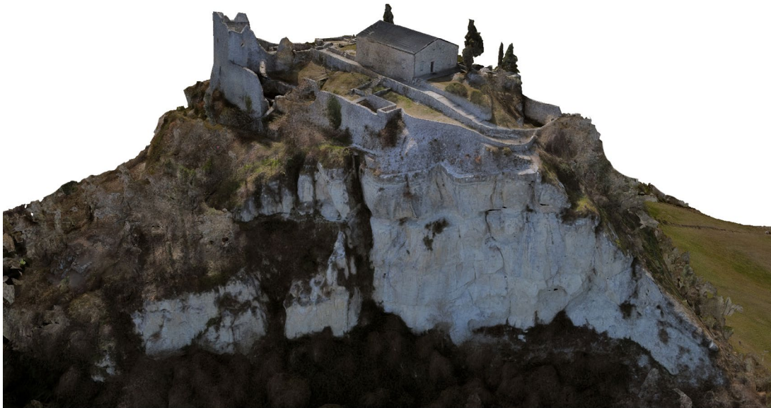
Fig. 11 - Two different views of the textured polygonal model obtained from the photogrammetric point cloud.
