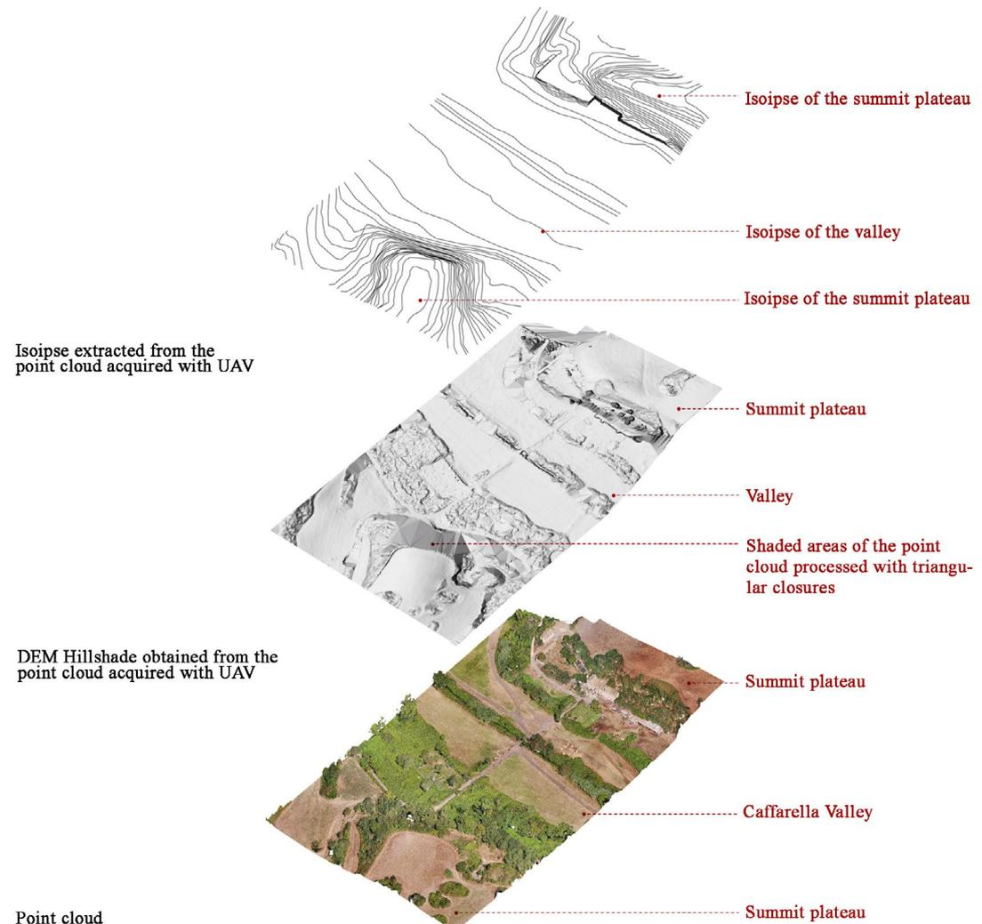
Fig. 12 - Point cloud, DEM Hillshade, and isoipse (elaboration by the author in Autodesk Autocad and ESRI - ArcGIS Pro 2.7)
