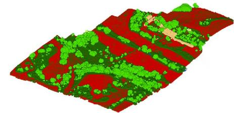
Fig. 9 - Classification of the point cloud in GIS (from top to bottom): Point cloud with unclassified RGB data; soil classification; building classification; and classification of plant elements (elaboration by the author in ESRI - ArcGIS Pro 2.7).
