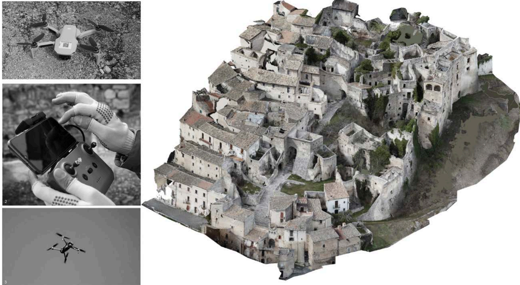
Fig. 5 - The aero photogrammetric survey: on the left the images of the instruments used; on the right the result of image processing..
