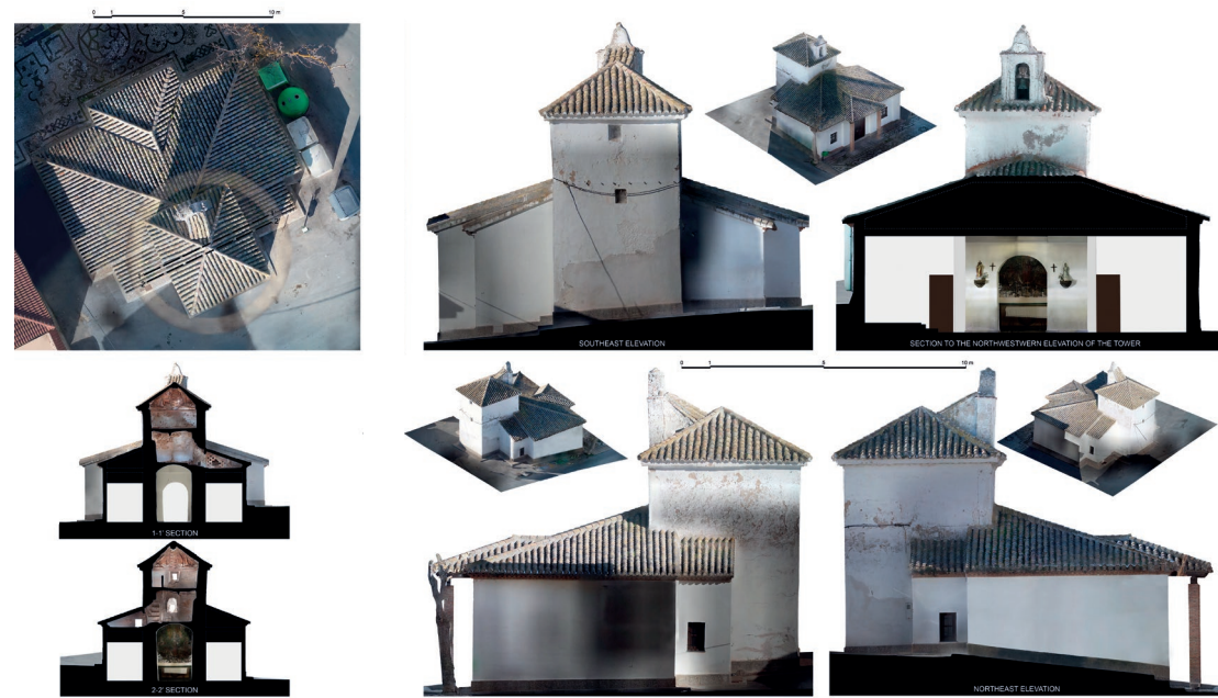
Fig. 7 - Graphical documentation of the Frontil Tower. Its remains are included in the bell tower of the Chapel of Nuestra Señora de la Esperanza (Loja).
