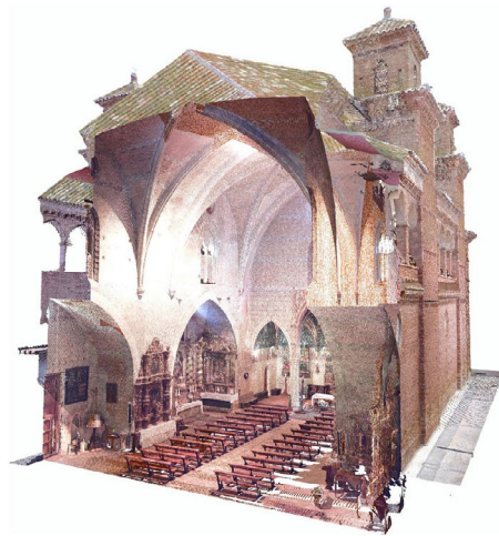
Fig. 6 - Three-dimensional geometric model obtained by combination of photogrammetric survey and laser scanning of the church of San Félix de Torralba de Ribota (Zaragoza). Prepared by Area of Architectural Graphic Expression of the University of Zaragoza.
