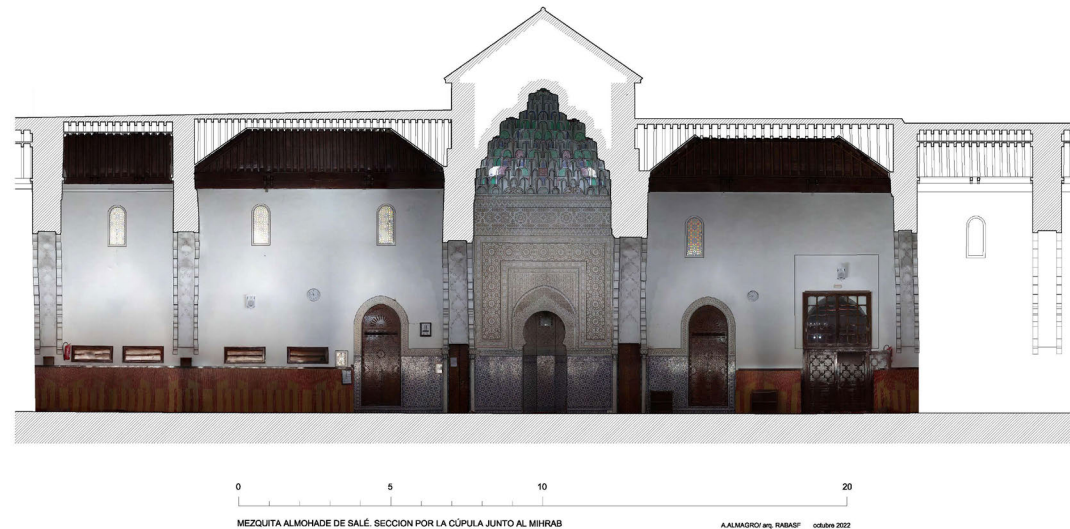
Fig. 5 - Cross - section with orthoimage of the Friday mosque of Sale (Morocco)
