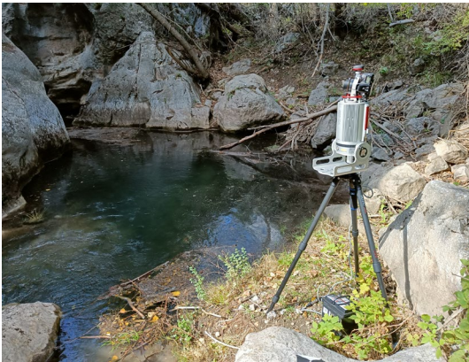
Fig. 8 - Riegl VZ400 laser scanner survey of the east side of the gorge
