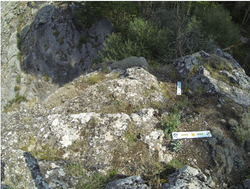
Fig. 3 - Scale bars to support photogrammetric surveys.
