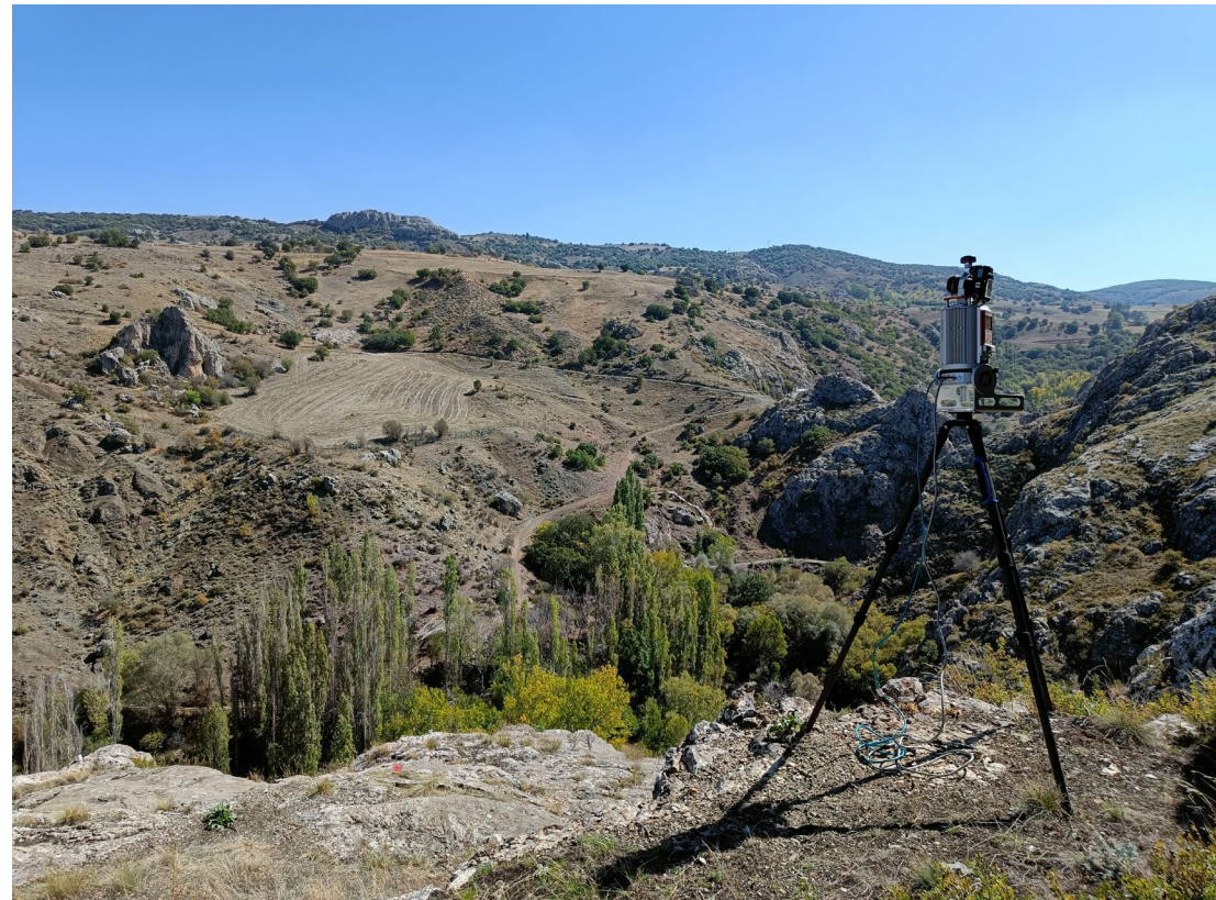
Fig. 2 - Riegl VZ400 laser scanner survey phases.
