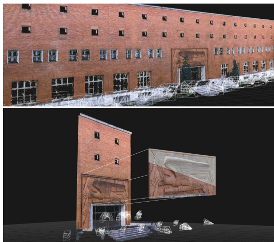
Fig. 12 - SfM photogrammetric acquisition phase and detail of the entrance
