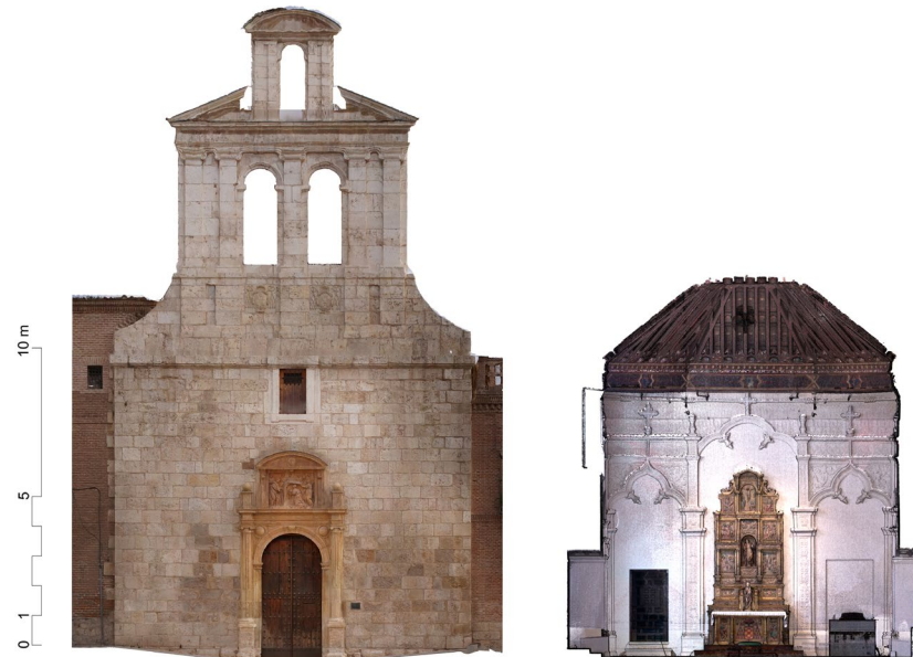
Fig.12. Survey of the façade by photogrammetric model (left) and of the interior by means of a laser scanner point cloud (right) of the chapel. By the authors.
