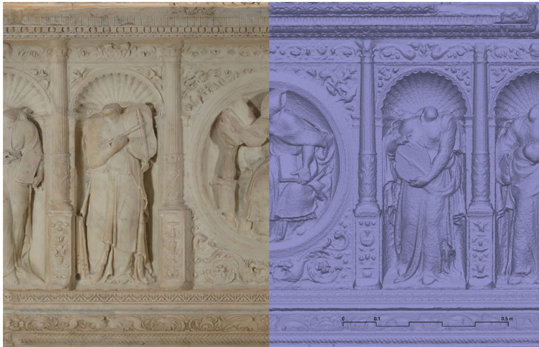
Fig.17. Detail of the photogrammetric model of the tomb of Cardinal Cisneros, in which the definition of the mesh can be observed. By the authors.
