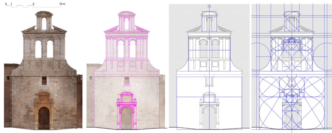
Fig.3. Study of geometry and proportions as an application of the survey. Elevation based on the golden ratio. By the authors.
