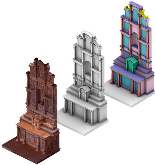
Fig.2. Volumetric analysis process from photogrammetric survey. By the authors.
