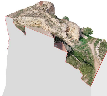
Fig. 20. Screenshot of the PointBox web viewer that allows to analyze and view the point cloud from any electronic device.
