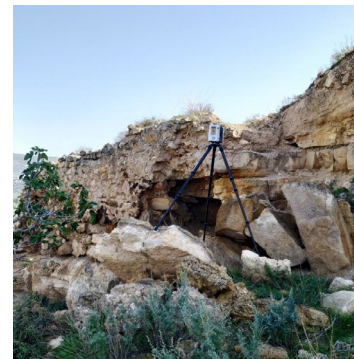
Fig. 7. Leica RTC 360 equipment during the scanning process of the fortress ruins.
