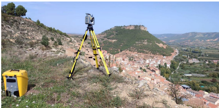
Fig. 7. Leica RTC 360 equipment during the scanning process of the fortress ruins.
