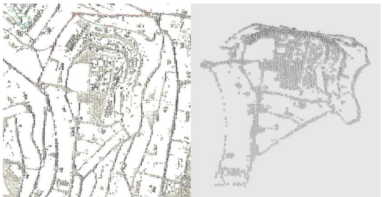
Fig. 7. Left: Lidar point cloud filtered (layer 2 'ground'). Right: 3D Lidar point cloud of pilot area exported to Rhinoceros.
