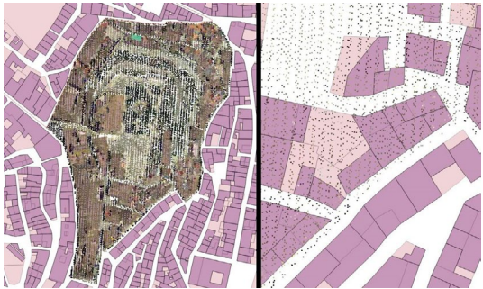
Fig. 6 Left: Lidar point cloud filtered (layers 2 and 6) and segmented to Pilot Area. Right: Density of Lidar point cloud.
