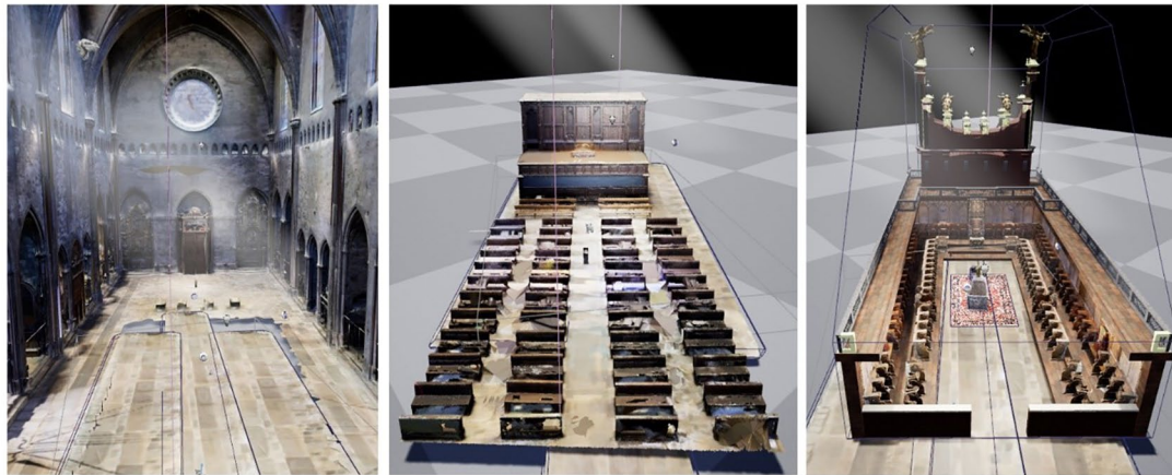
Fig. 11 -The empty Cathedral precinct, current situation, and model generated from the photogrammetric captures. (Own elaboration)
