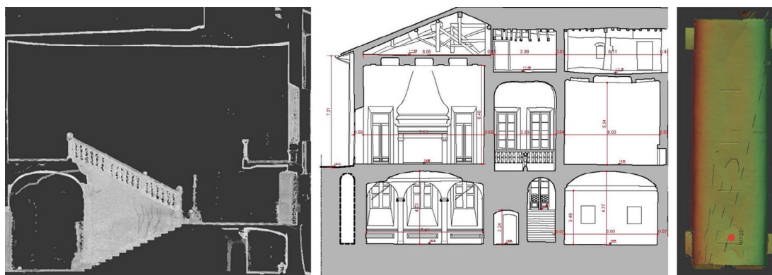
Figure. 7 Villa Cicogna Mozzoni: the laser scanner survey of the vault covering the great hall of honor showed the deformation of the wooden structure hanging, irregular in its course, toward the window (drawings: arch. Anna Urso).
