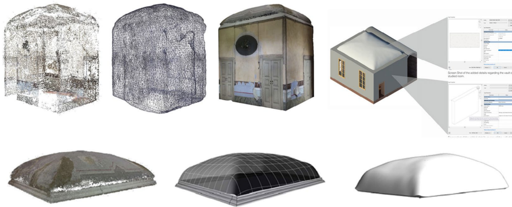
Figure. 4 From point clouds obtained photogrammetrically to the HBIM model of a vaulted room.
