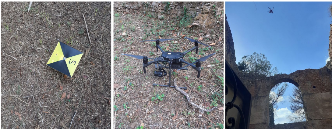
Fig. 3. Acquisition of the Mausoleum of Sant'Urbano using a DJI Matrice 210 V2 UAV with a Zenmuse X5S camera (photo by the authors, September 2022).
