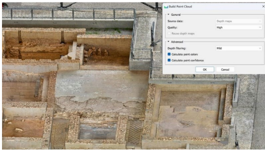
Fig. 12 - Parameters used in the research to obtain the dense point cloud.
