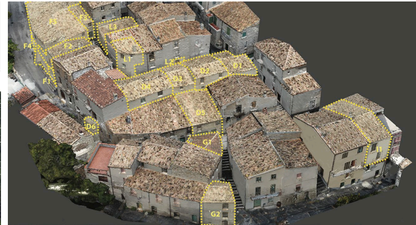
Fig. 5 - Semanticisation and reconstruction of the urban fabric from a drone photogrammetric acquisition. Image above by M. Canciani, M. D'Angelico "A methodology for survey, documentation and virtual reconstruction of historical centers in a seismic area: the case study of Arquata del Tronto". Image below by C. Costantino, A. C. Benedetti, G. Predari, "UAV Photogrammetric survey as a fast and low-cost tool to foster the conservation of small villages. The case study of San Giovanni Lipioni". (Proceedings of the 2nd D-Site conference).
