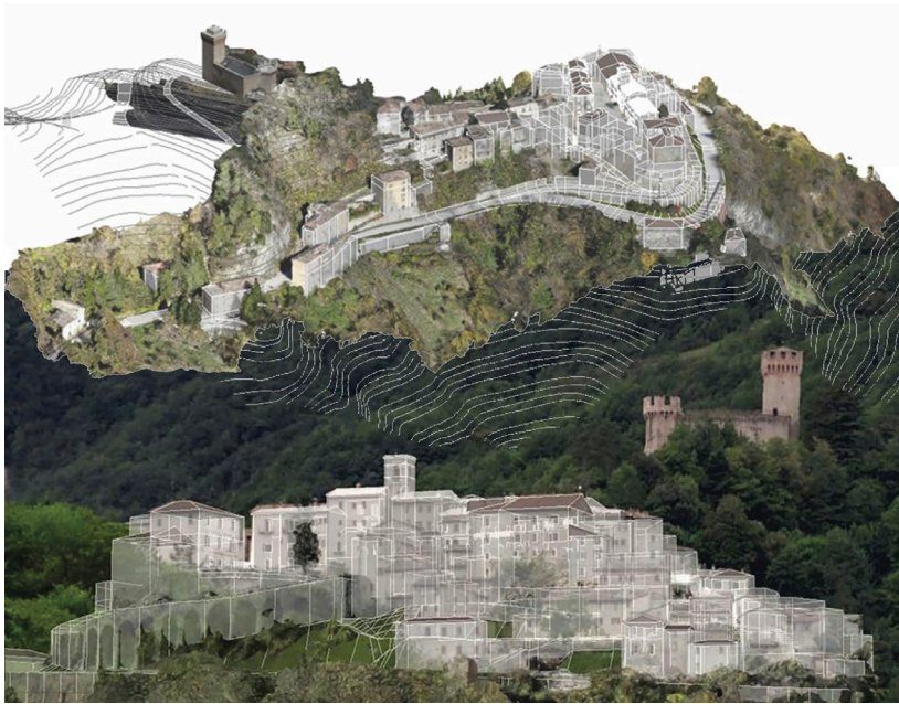
Fig. 5 - Semanticisation and reconstruction of the urban fabric from a drone photogrammetric acquisition. Image above by M. Canciani, M. D'Angelico "A methodology for survey, documentation and virtual reconstruction of historical centers in a seismic area: the case study of Arquata del Tronto". Image below by C. Costantino, A. C. Benedetti, G. Predari, "UAV Photogrammetric survey as a fast and low-cost tool to foster the conservation of small villages. The case study of San Giovanni Lipioni". (Proceedings of the 2nd D-Site conference).
