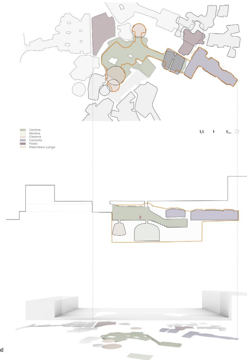
Fig. 7 - Plan, section and three-dimensional view of the set of spaces excavated before the formation of the Palombaro Lungo. 1870. In dark green the cantina, in light green the neviera adjacent, in purple the conceria and in pink the cisterne, the orange line corresponds to the contour of the volume resulting from Palombaro Lungo.
