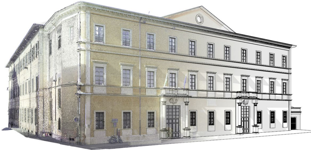
Fig. 8: The point cloud and the HBIM model obtained from the scan-to-BIM process
