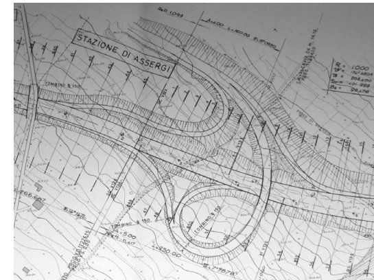
Fig.2 - Above: S.A.R.A.. Project of the highway L'Aquila-Villa Vomano. Detail of the exit to Assergi, close to the Gran Sasso. 1971, ASAQ 9 BN 10 116
