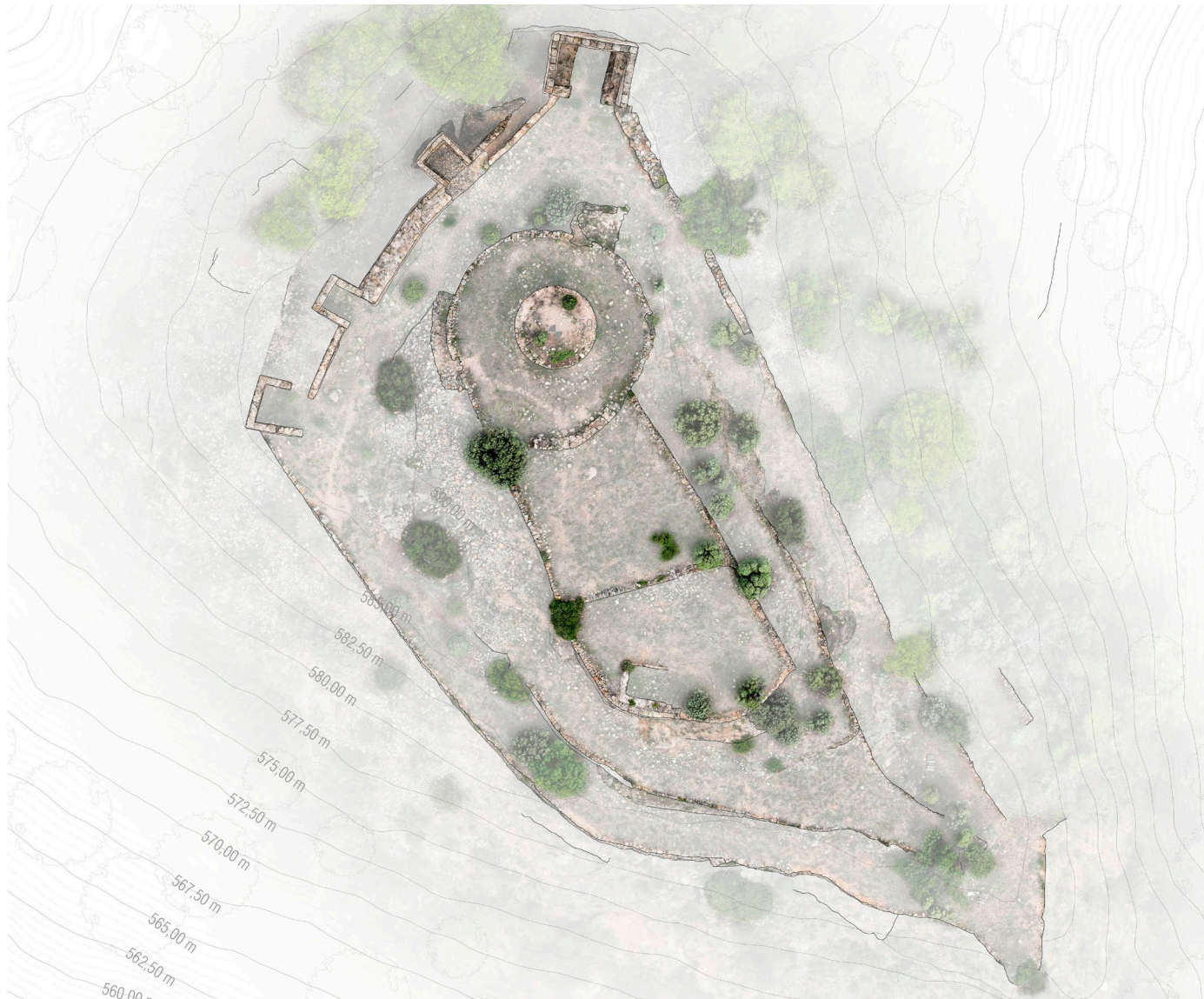
Fig. 7.8 - Layout and detail of the tower of Alcudia de Veo Castle (Alcudia de Veo, Castellón, Valencia). Layout obtained from the 3D photogrammetric model. The flight was carried out with a DJI Mavic 3E drone +RTK, with the aim of obtaining the scaled graphic documentation. The layout is in 1/200, so the required resolution for printing at 300 dpi was 17 mm/pix, and the tower in 1/50, and the required resolution for printing at 300 dpi was 4.3 mm/pix (Pablo Rodríguez-Navarro, Teresa Gil-Piqueras, Anna Pérez Vila).
