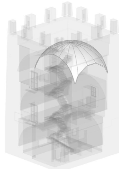
Figure 11. Staircases (a) and sail vault (b) of the Rame tower modelled from the point cloud with Edificius by ACCA Software S.p.a. (García-León et al., 2023).
