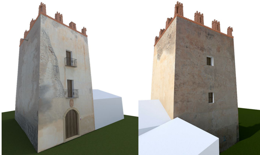
Figure 12. Render of the Rame Tower HBIM, south view (a) and north view (b) made possible only with the version BIM 3 (e) of the ACCA's BIM authoring software "Edificius".
