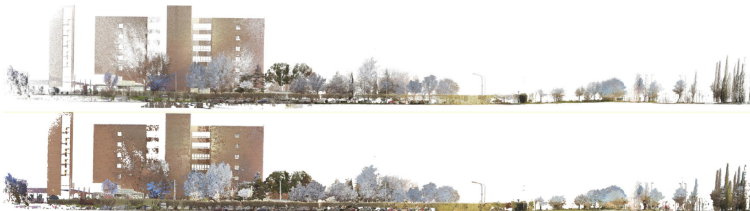
Fig. 13: Comparison of rendered elevations from Cloud Compare. Original elevation (top) and elevation scaling the RGB points (bottom). By the authors.
