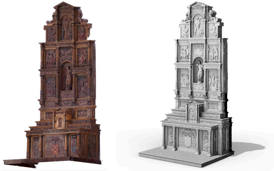
Fig. 4 - Model of the Altarpiece. Mesh from Photogrammetry (left) and modified mesh with corrections (Right). By the authors
