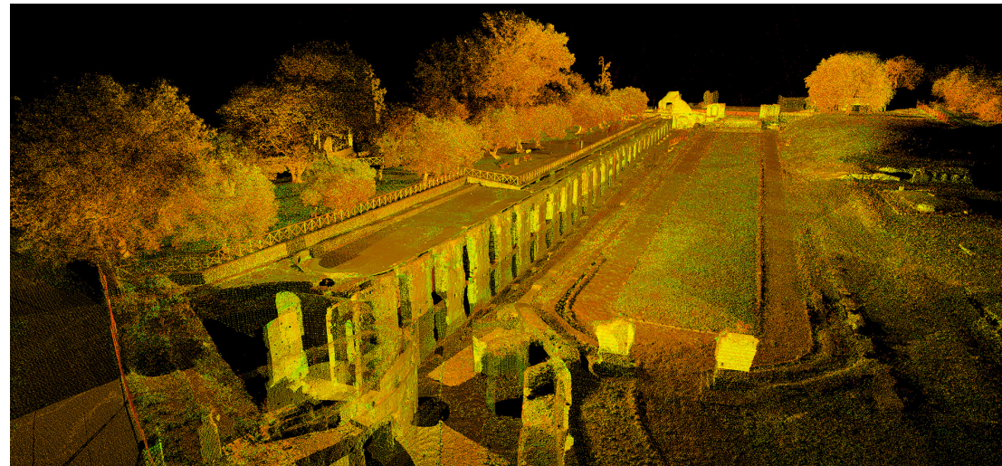
Fig. 11 - Bottom: Perspective view of the registered point cloud from the terrestrial laser scanner campaign of the area. Point cloud registration: S. Bertacchi.
