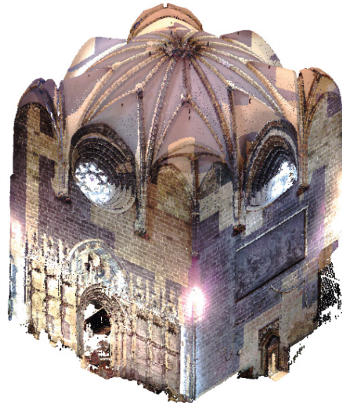
Fig. 6 - Point cloud of the interior envelope of the Chapel of the Holy Chalice and segmentation using RANSAC.
