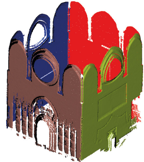
Fig. 6 - Point cloud of the interior envelope of the Chapel of the Holy Chalice and segmentation using RANSAC.
