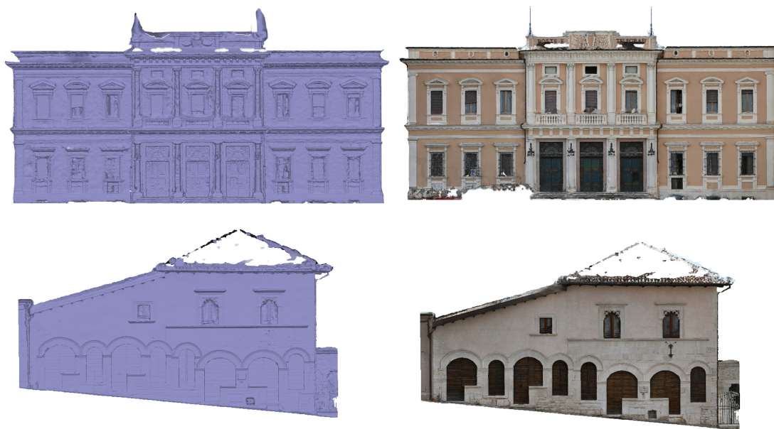
Fig. 5 - Output of the photogrammetric survey of "Poste e Telegrafi" palace (top) and "Cancelle" (bottom). On the left mesh in solid view, on the right model textured.
