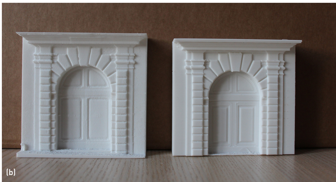
Fig. 12 – Comparison between the prototype obtained from the photogrammetric model, on the left, and the one obtained from the NURBS model, on the right: (a) scale 1:100; (b) scale 1:50.
