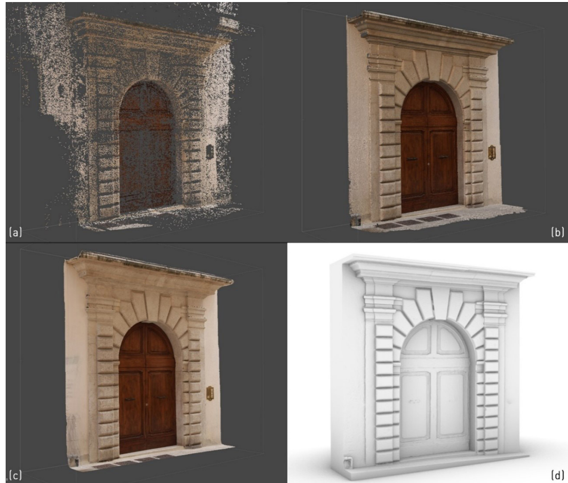
Fig. 4 – The elaboration of the photogrammetric model: (a) the sparse cloud; (b) the dense cloud; (c) the texturized mesh; (d) the model ready for the export in .stl format and the importation in the slicer software.
