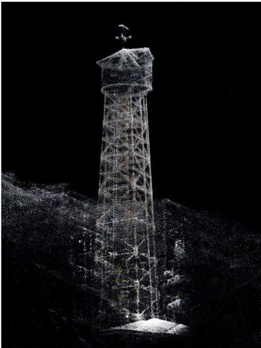
Fig. 2 - Processed Photogrammetry Point Cloud. Rendered in Reality Capture – Credit Sam Smith - WOODS
