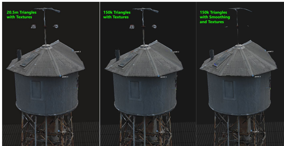
Fig. 7 - Colonial Ammunition Shot Tower. Comparison of textured mesh model after simplification and texture reprojections. Credit – Sam Smith - WOODS
