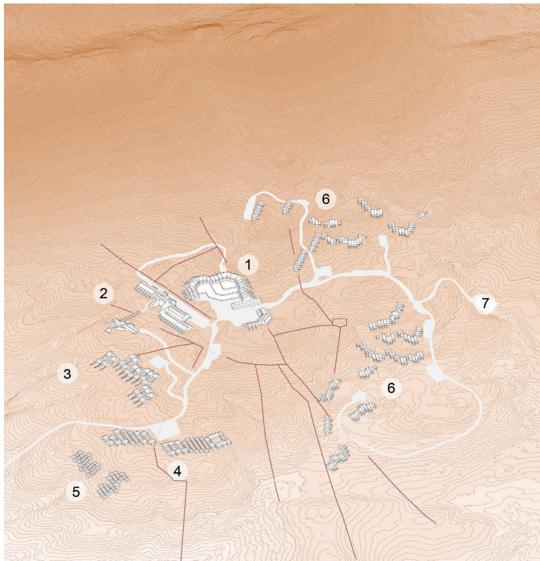
Fig. 6 - Stazzo Pulcheddu's isometric. [1] Plaza and perimetral buildings/ [2] Residence/ [3] Patio- houses 1ª phase, 90 sqm/ [4] Patio- houses 2ª phase, 70 sqm/[5] Patio- houses 3rd phase, 60 sqm/ [6] Grouped single-family houses/ [7] Sports zone. Drawing made by the author.
