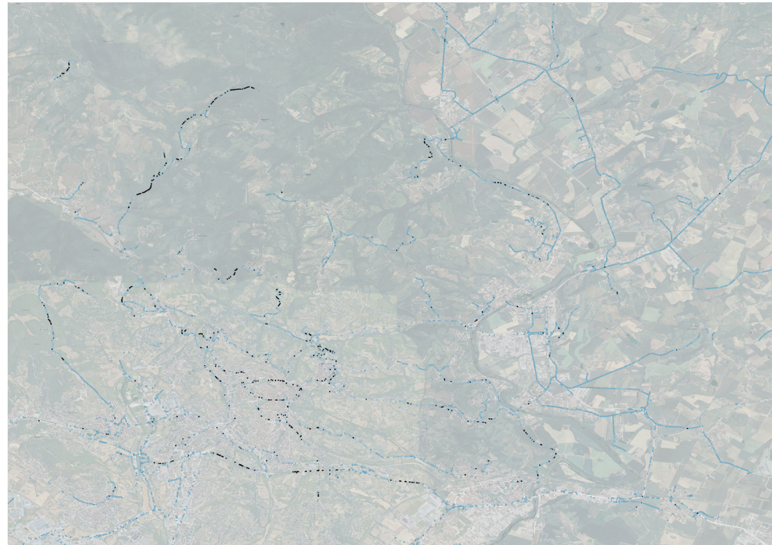
Fig. 3 Sky View Factor (SVF) distribution in Perugia for 2023. The graph shows an average SVF of 0.27, with central areas (in black) displaying limited sky visibility due to the high density of buildings, while peripheral areas (in light blue) offer better visibility. This contrast highlights the impact of urban density on the perception of openness in the urban environment.
