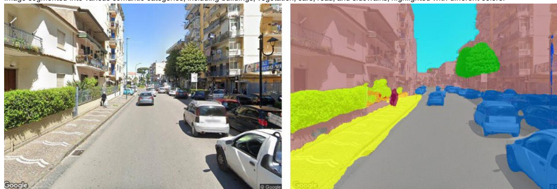
Fig. 1 Example of semantic segmentation applied to an urban image: on the left, the original image captured from Google Street View; on the right, the same image segmented into various semantic categories, including buildings, vegetation, cars, road, and sidewalks, highlighted with different colors.
