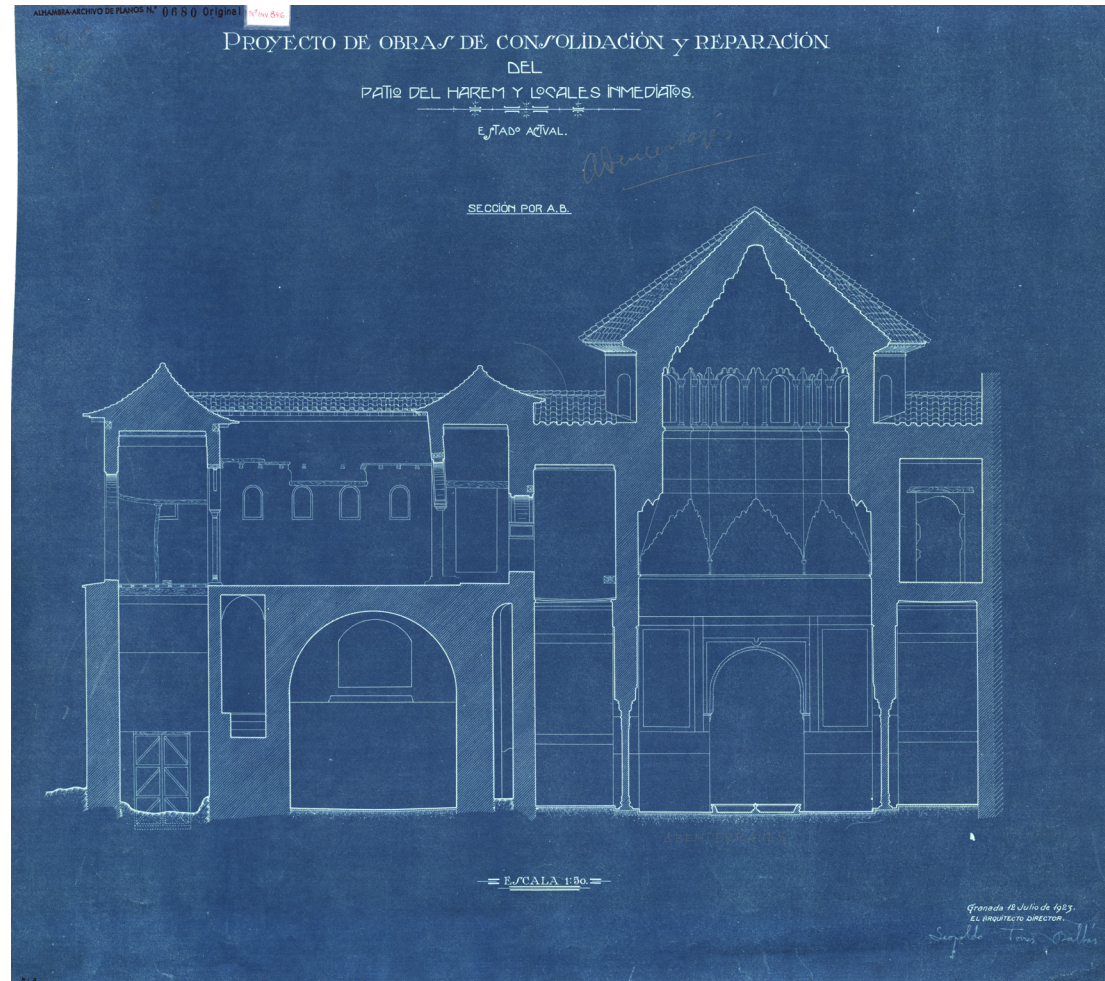
Fig. 7 - Project for consolidation and repair works of the Patio del Harén and adjacent areas. Current state, Granada, July 1923, M. López Bueno and L. Torres Balbás. Copy, paper, cyanotype, 54 x 60 cm (APAG / Plan Collection / P-000846).
