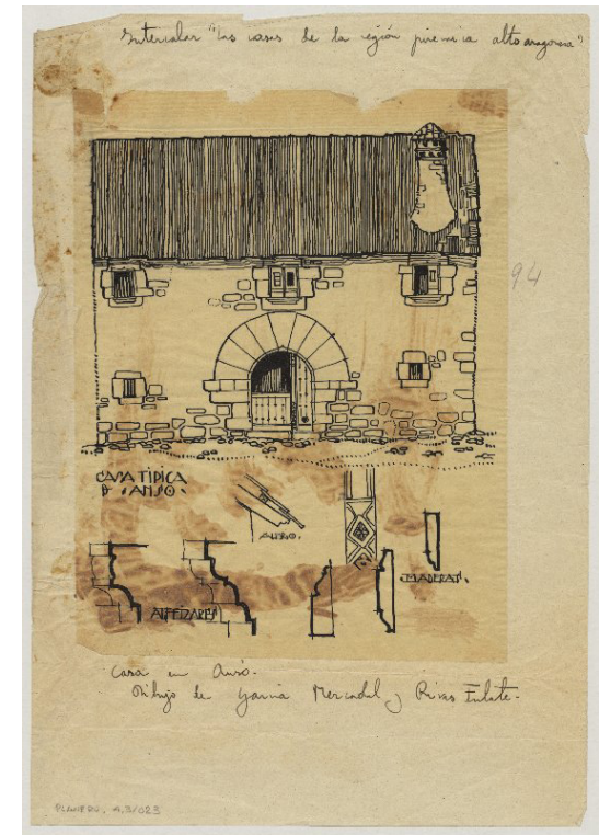
Fig. 1 - Elevation drawing of a two-story house in Anso, with details of cornices and eaves, c. 1922, F. García Mercadal and J.M. Rivas Eulate. Tracing paper, ink, 17.4 x 20 cm, mounted on paper measuring 21.6 x 31.5 cm (AGRM, PLANERO, 4/3,023).
