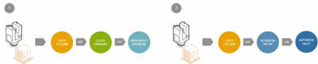
Figure 4 - From point cloud to BIM environment importing process diagram - original drawing
