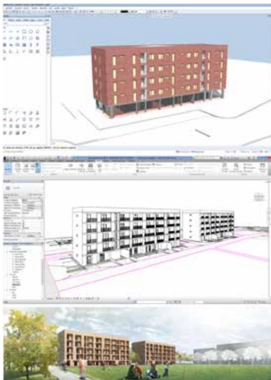
Figure 6 - Compagnoni Fenulli District in Reggio Emilia: different visualization of different models aimed at Facility Management - BIM authoring in different software environment and render
