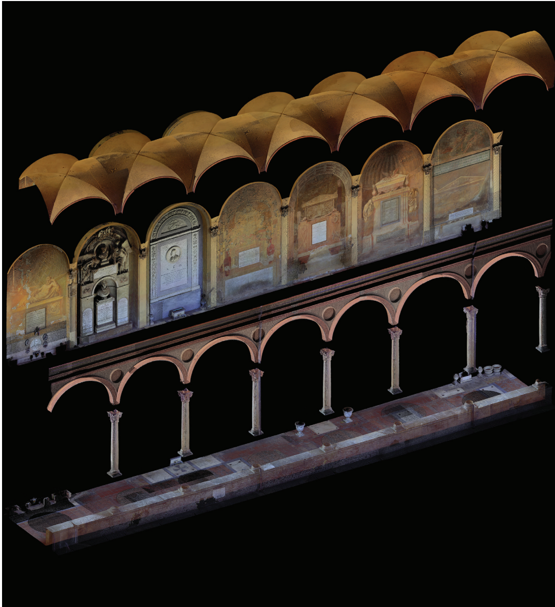
Figure 2 Semantic segmentation of the architectural path in the cloister III of the Certosa di Bologna.
