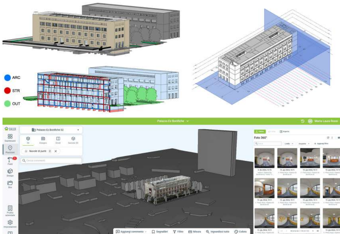
Fig. 18_ Civil reconstruction model (Autodesk Revit BIM application) managed together with other information models and documentation in the open platform (Dalux).
