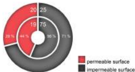
Fig. 13 - Diagram of the impermeable surfaces increasing from 1975 to 2025.
