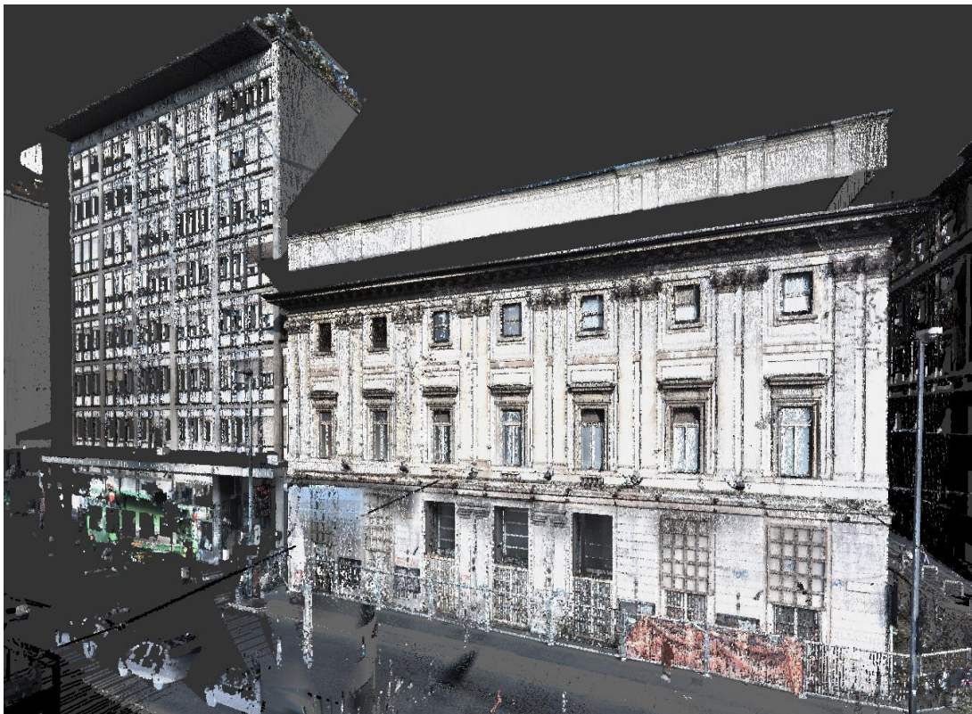
Figure 9. Survey with laser scanning of the outside of the Teatro Lirico in Milan (inthefold.autodesk.com).
