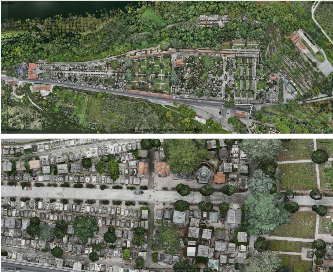
Fig. 13 - Model of the Monumental Cemetery of Perugia: images of the point cloud generated through aerial photogrammetry, developed in collaboration with ITC-CNR of L'Aquila, Italy.
