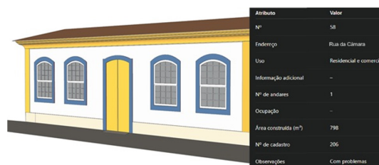
Fig. 17 - 3D BIM model of the property located at Câmara Street, in the historic centre of Tiradentes. Source: Prepared by the authors (2025).
