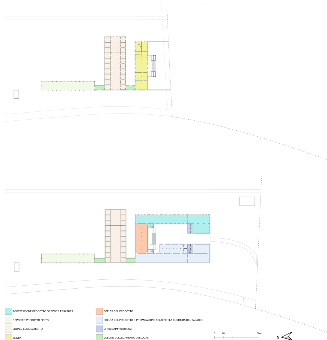
Fig.04 - Tobacco Factory in Presenzano: plans at elevations 143.2 and 146.0 meters extracted from the BIM model showing the functional areas of the factory (model by the Authors).
