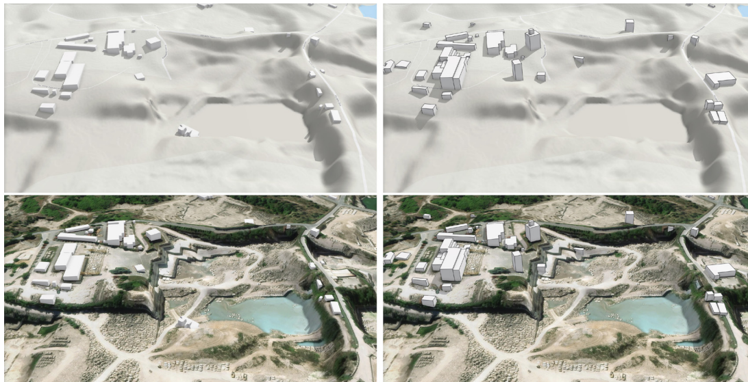
Fig. 4 - Comparison between the OpenStreetMap 3D building database (left) and ESRI (right). The number, footprint, and heights of the buildings are different.
