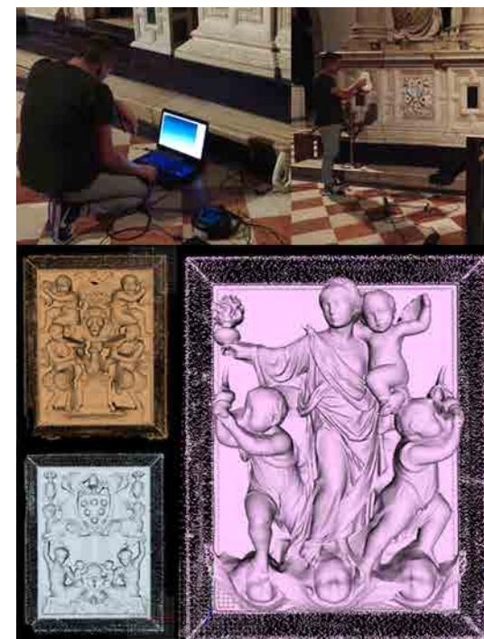
Fig. 8: The instrumental survey carried out by Scanner 3D Artec Eva: snapshot of the campaign and some processed scans of the Holy House panels.
