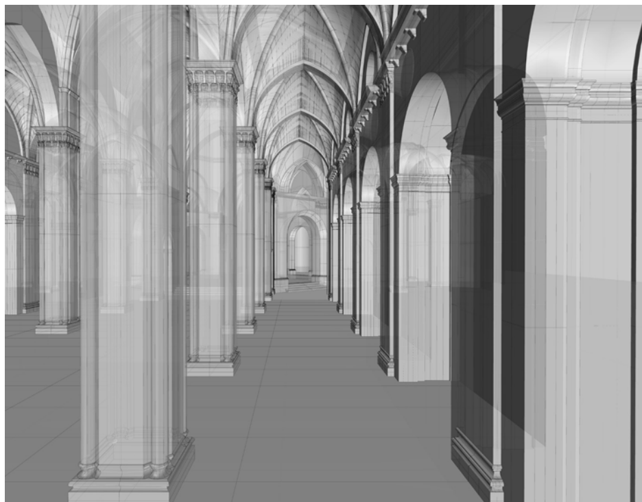
Fig. 9: NURBS model of the Basilica in its current state: perspective view of the side aisle.
