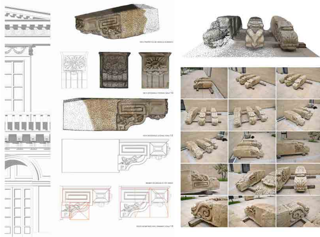
Fig. 12. Bourbon Municipal Theatre. Application of Augmented Reality and repositioning in the three-dimensional model of the finding number XIX25 Limestone shelf with classical meander decoration.
