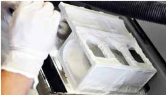
Fig 15. 3D printing and final cleaning of the chalk prototype.
