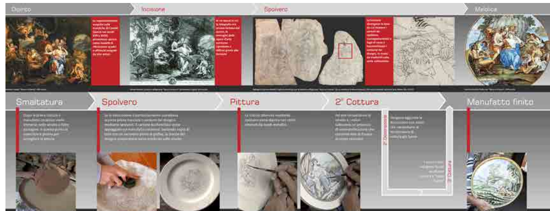
Fig 3. Mimic diagram of processing steps of majolica.
