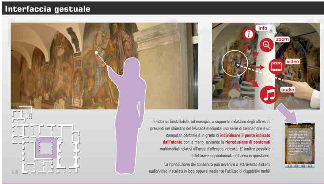
Fig. 15. Using gestural interfaces integrated with MOCAP techniques for the computerization of fresco of the cloister.
