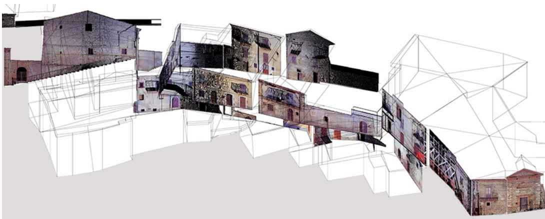
Fig.13 Some photoplanes placed on the 3D model in wireframes of the historic nucleus: Via Umberto I and piazzetta Sant'Antonio (SCUT)
