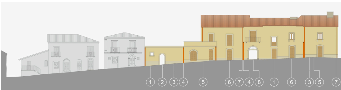
Fig.14 Extract from the Reconstruction Plan: Proposed external arrangement of the Baron's palace (SCUT): 1) stone or stucco frames, 2) re-opening the walled portal, 3) apricot basement socket, 4) best of iron corten and body Integrated light fixture, 5) traditional colored plaster paste, 6) wooden fixtures, 7) copper plummet, 8) baronial palace gallery.
